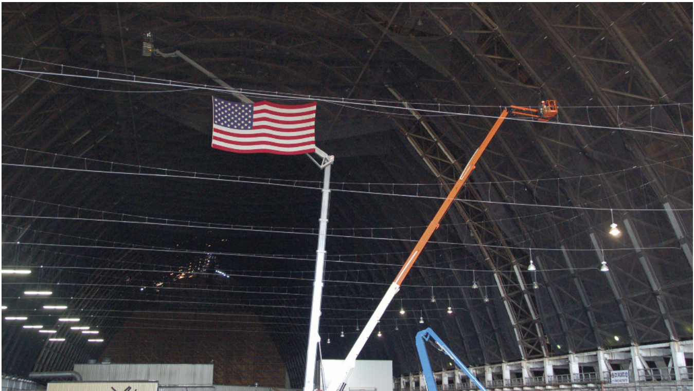
The 300 ft. Bronto S-90 lift on left, next to 135 ft. JLG boom lift on right.
